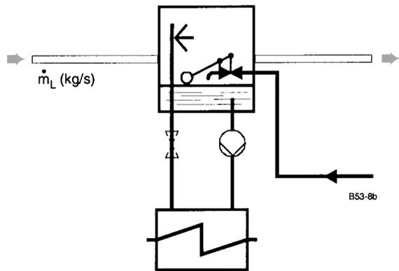
Fig. 3-8b Humidifying at a variable water temperature
