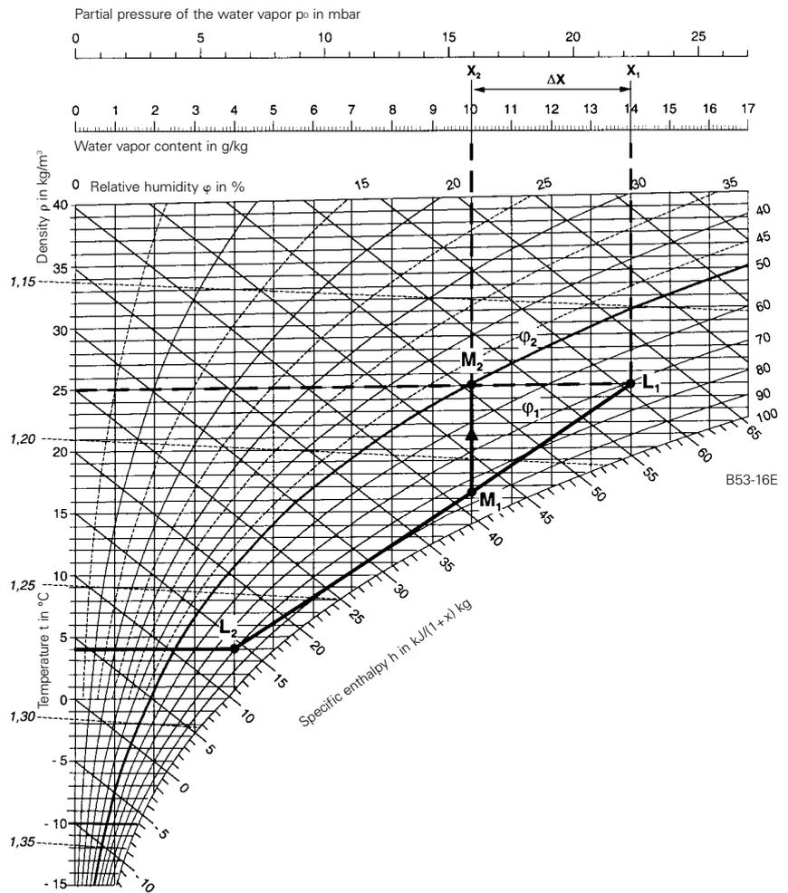
Fig. 3-16 Air drying by mixing and reheating
