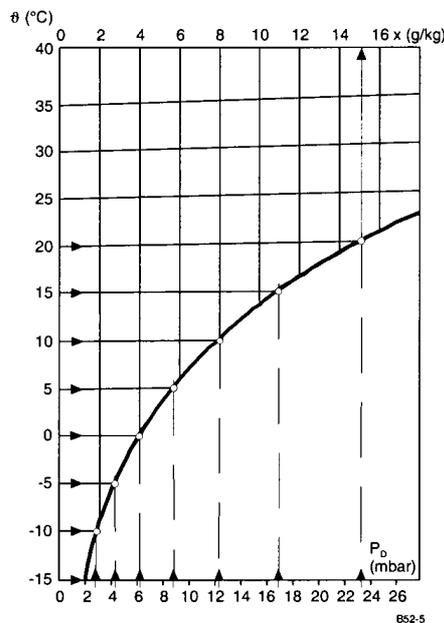
Fig. 2-5 Saturation pressure  $p_s$
