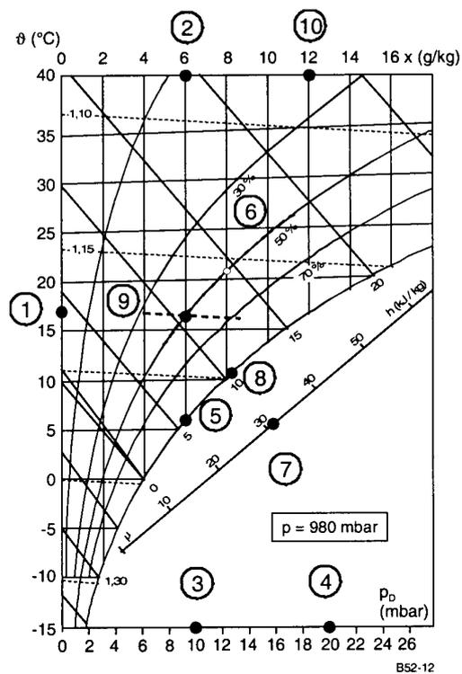
Fig. 2-12 Defining the air state using ten variables
