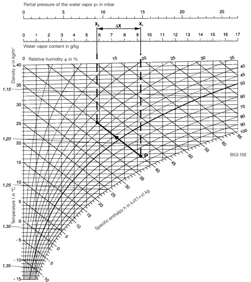
Fig. 3-15 Drying air using the absorption method
