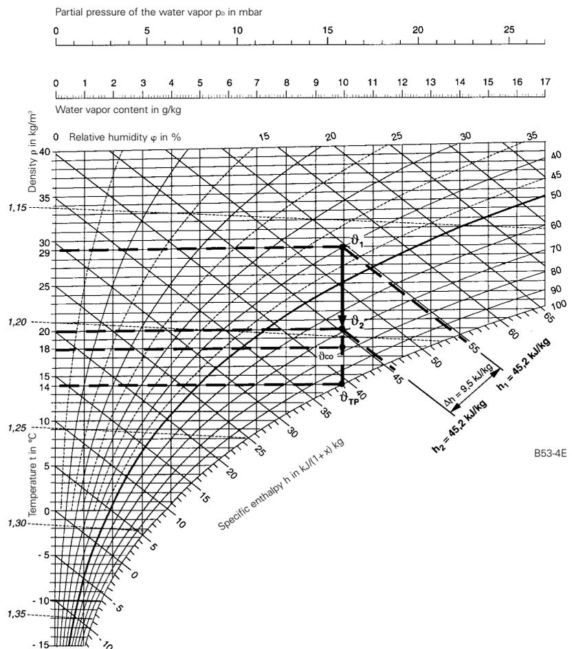
Fig. 3-4 Air cooling using a dry cooling surface
