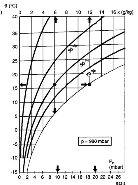
Fig. 2-8 Determining seven variables for a given point
