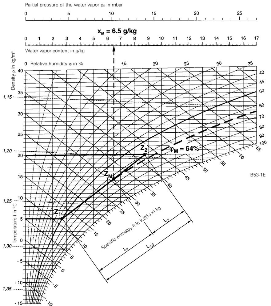
Fig. 3-1 Mixing of air flows  $Z_1$  and  $Z_2$
