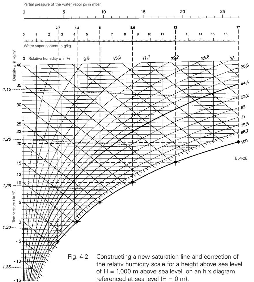
Fig. 4-2 Constructing a new saturation line and correction of the relative humidity scale for a height above sea level of  $H = 1,000$  m above sea level, on an  $h, x$  diagram referenced at sea level ( $H = 0$  m).
