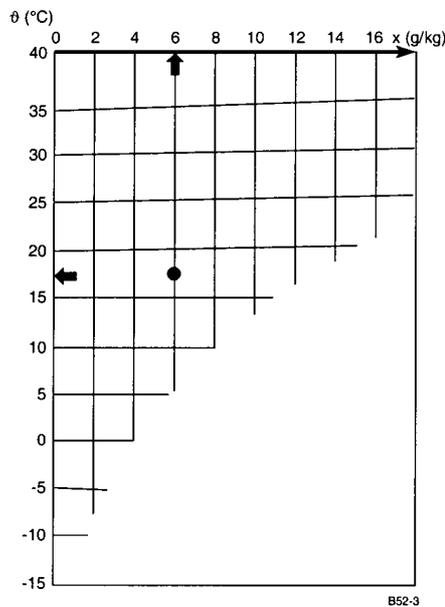
Fig. 2-3 Water content  $x$  and air temperature
