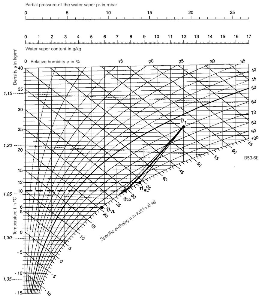
Fig. 3-6 Actual cooling process for a wet cooling surface
