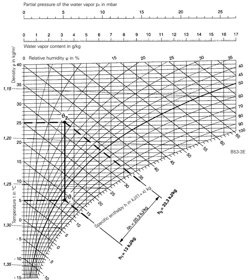
Fig. 3-3 Heating the air
